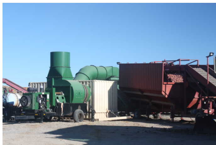
Trucks dump their field loads into the red tub. The green vacuum pump sucks the potatoes up on to a conveyor belt while separating loose dirt, rocks and vines into a separate box for recycling back to the fields.
